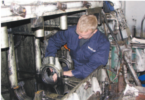
Preparing for Line Boring
